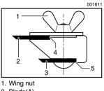
First, loosen the two wing nuts on the holder and insert the blades (A) and (B), so that they contact the sides (C) and (D). Then tighten the wing nuts.
