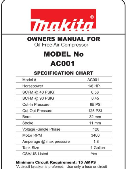
\*A circuit breaker is preferred. Use only a fuse or circuit breaker that is the same rating as the branch circuit the air compressor is operated on. If the air compressor is connected to a circuit protected by fuses, use time delay fuses.
