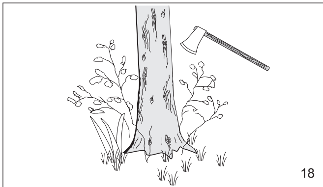
First clear the tree base and work area from interfering limbs and brush and clean its lower portion an axe (see Fig. 18).
