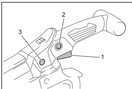
► 1. Switch trigger 2. Lock button 3. Trigger-lock button
